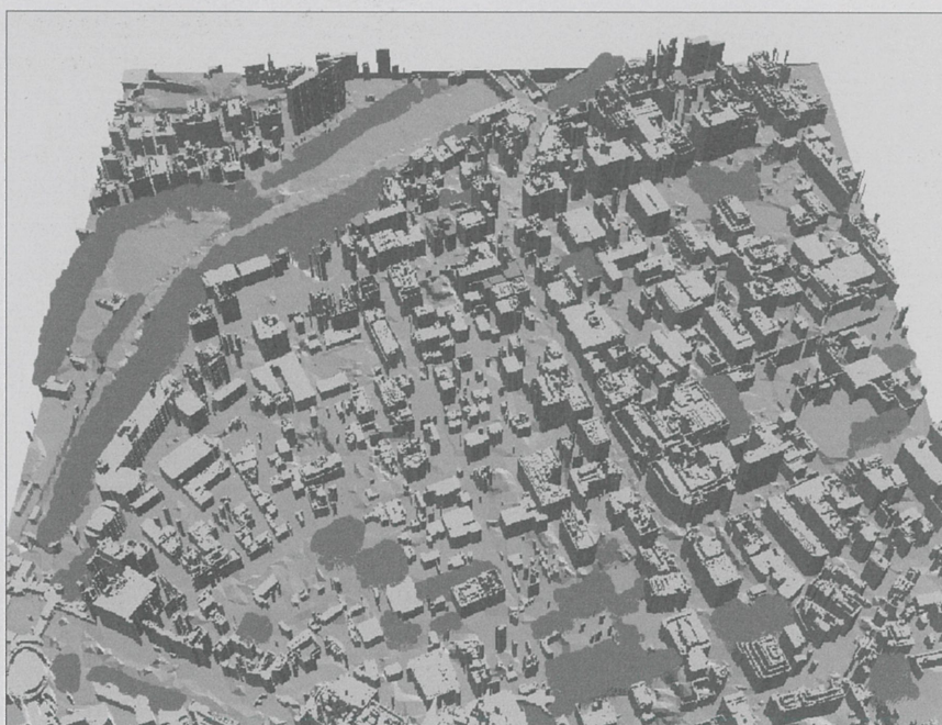
Three-dimensional expression of bird's-eye view of a city made by laser scanner
