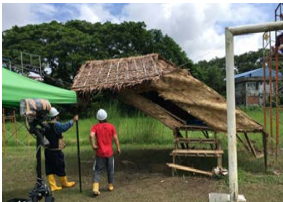
Pull-down testing of Bamboo structured house
