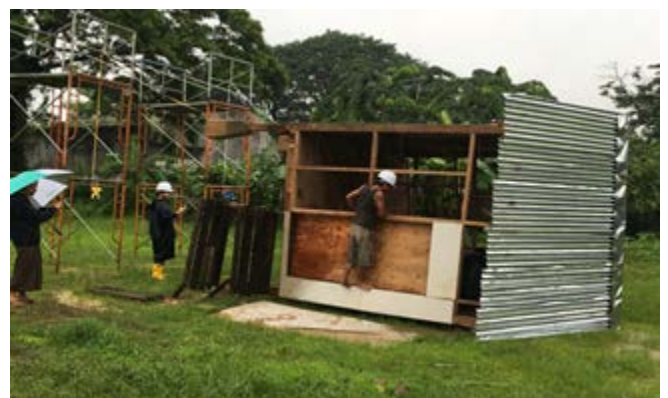
Pull-down testing of Bamboo structured house
