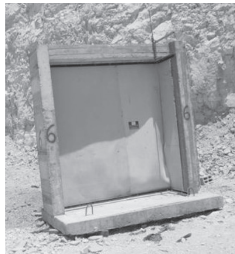
Figure 16: Post-detonation picture of threat side and structure interior side. Slight anchor loading due to placement of charge 50cm off the corner
