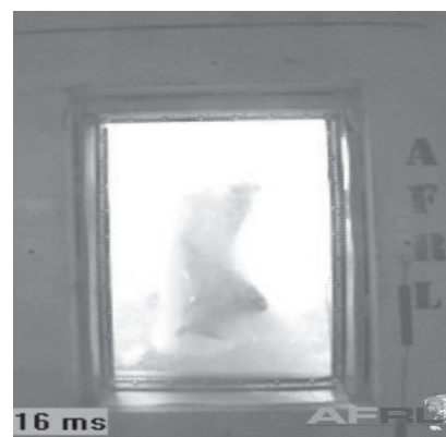
(f) 116ms EASF glazing pulverized no fragments or shards inside structure.
