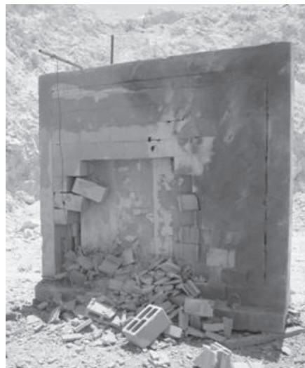
Figure 16: Post-detonation picture of threat side and structure interior side. Slight anchor loading due to placement of charge 50cm off the corner
