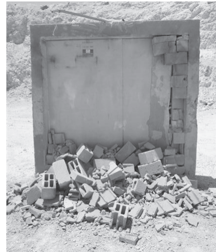
Figure 15: Post-detonation picture of threat side and structure interior side. No evidence of anchor loading.
