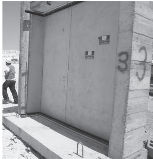
Figure 14: Post detonation pictures of threat side and building interior side. No debris on interior side and no evidence of anchor loading
