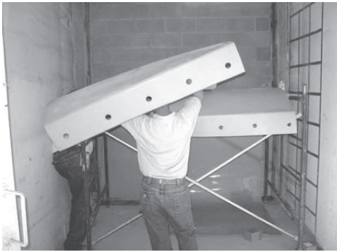
Figure 9: Shield Wall Panels installed 33 feet from detonation on ungrouted masonry infill wall
