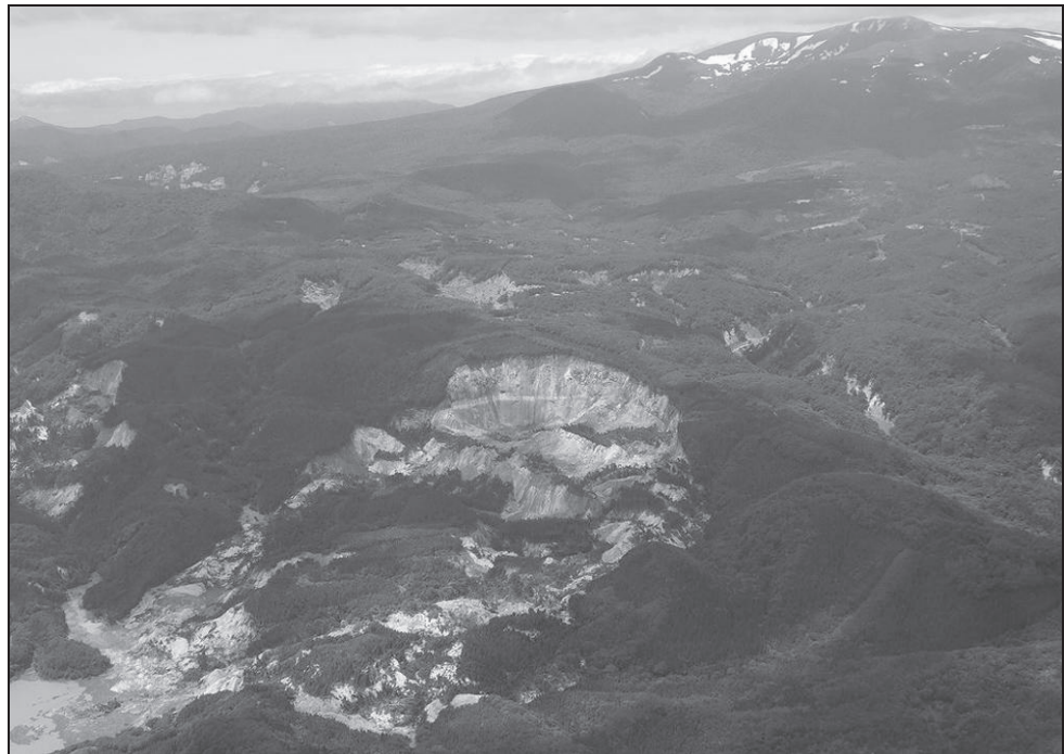
Figure 2: Landslide at Aratosawa dam: Aerial photo of the largest landslide with Kurikoma Volcano rising behind. The terrain here is suggestive that similar landslides have been reactivated.
