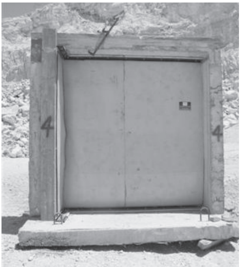
Figure 12: Series of Life Shield Wall Panel tests against 4 kilograms of TNT at 50, 70, and 120 centimeters in fragmentation casing
