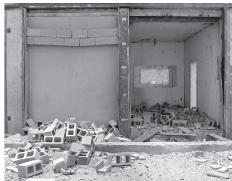
Figure 11: Life Shield Wall Panels intact on the left side, control fails catastrophically on right side
