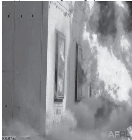
(d) EPFS Repelling Entire Window Mass Including Shards
