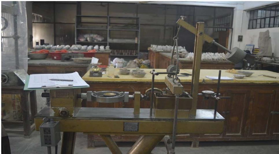
**Figure 7.2. Equipment of Direct Shear Test.**
