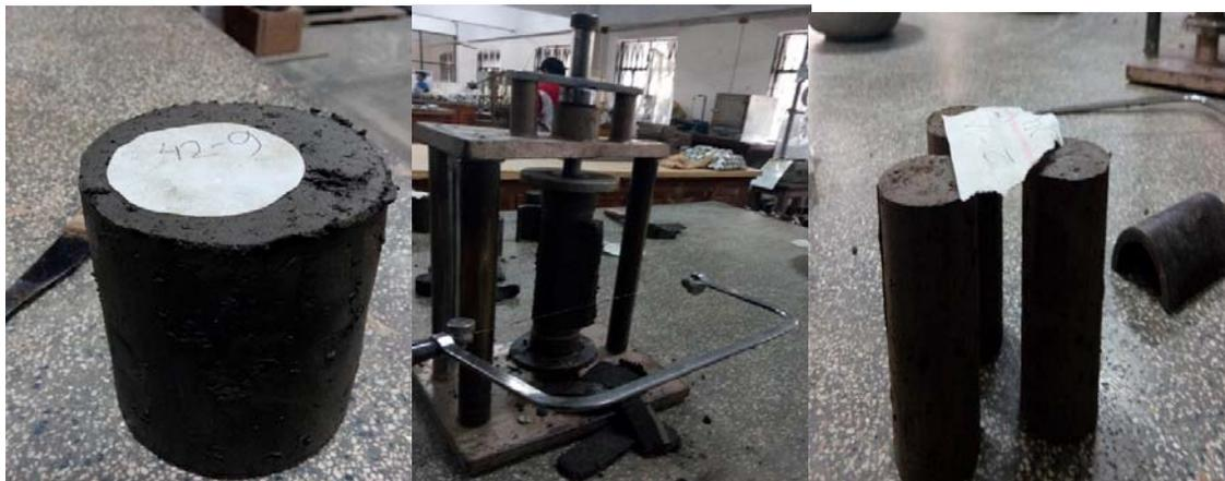
Fig 5.14 : Preparation of samples for unconfined compression test from compacted mold
