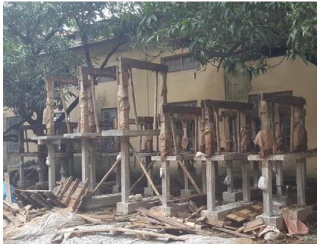
Figure 4: Prototype models of Bangladeshi RCC structures to be tested on shaketable
