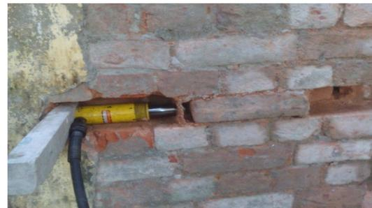
Figure 11: Direct Shear Test
