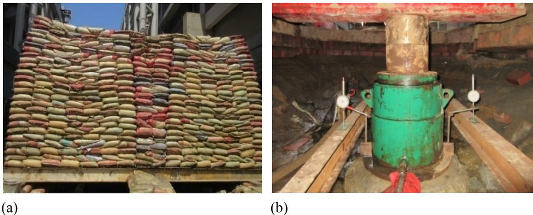
**Figure 7: (a) Static Loading System on top of a JGC and (b) Hydraulic Jack and dial gage setup**
