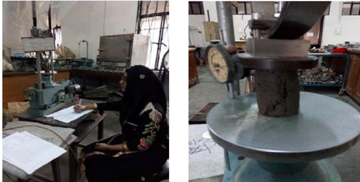
Fig 5.15: (a) Recording data for unconfined compression test (b) Failure of sample
