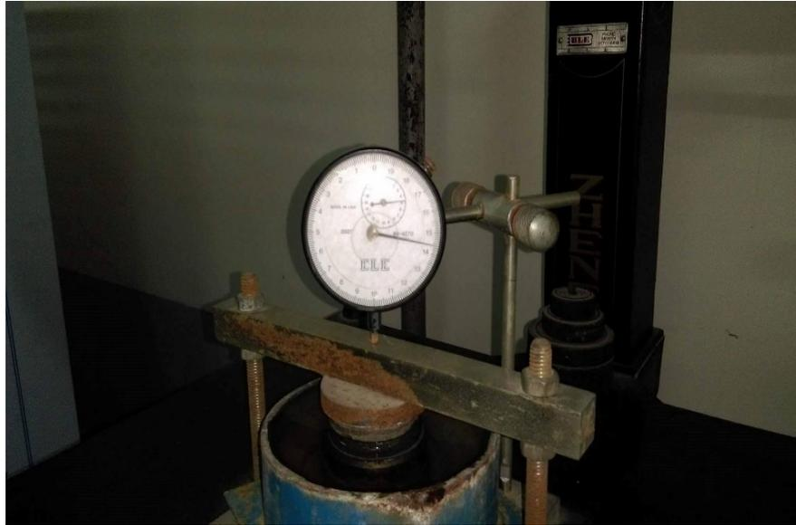
Fig 5.17: Consolidation test Apparatus
