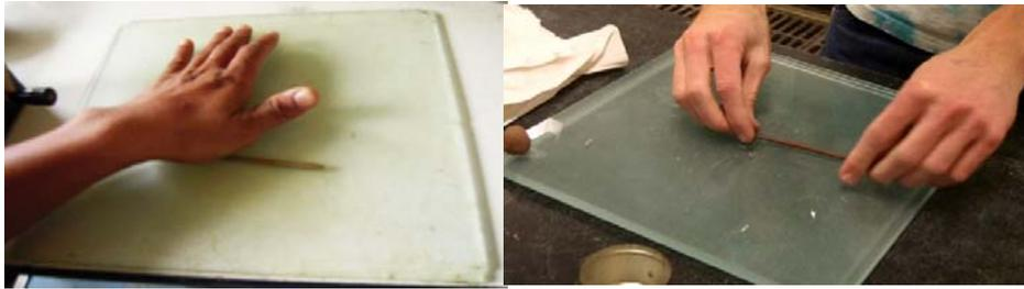
Fig 5.11 : Plastic Limit test
