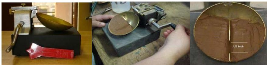
Fig 5.12: Liquid limit test with casagrande apparatus
