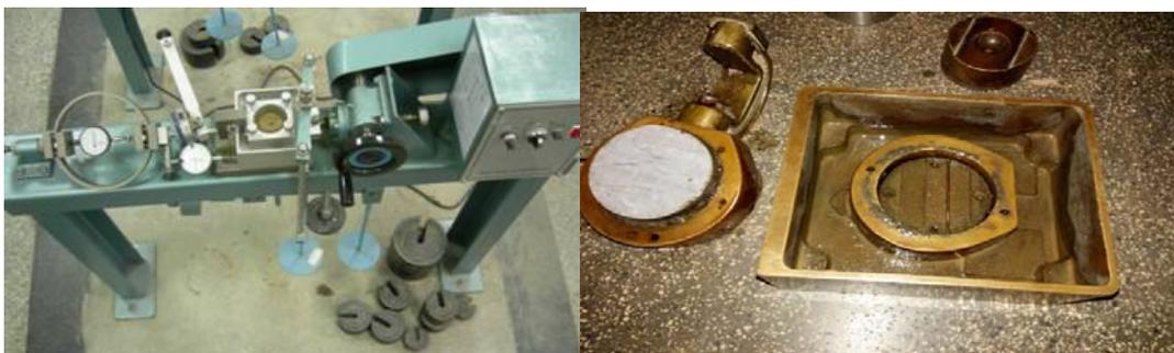
Fig 5.16: Direct shear apparatus with shear box
