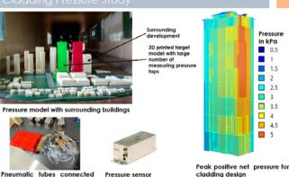
The cladding pressure on façade can be measured in wind tunnel and scaled to full scale pressure after combining with the local wind climate.
