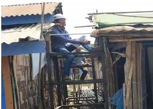
Pull—down test experiment in slum area of Yangon
