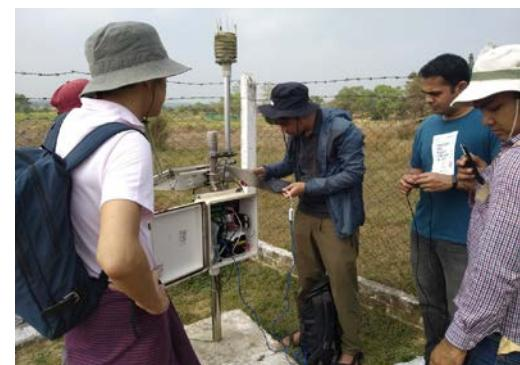
Maintenance and solving data transmission problem at Automatic Weather Station (AWS) at Zaung Tu Weir
