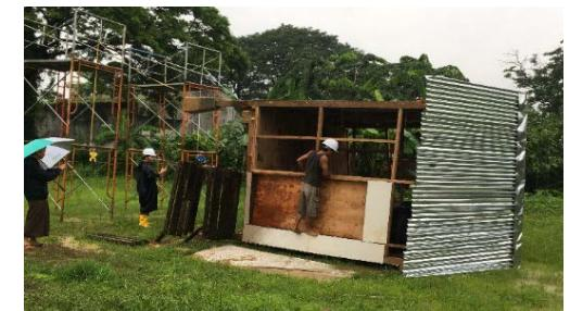
Pull down testing of timbered structure house
