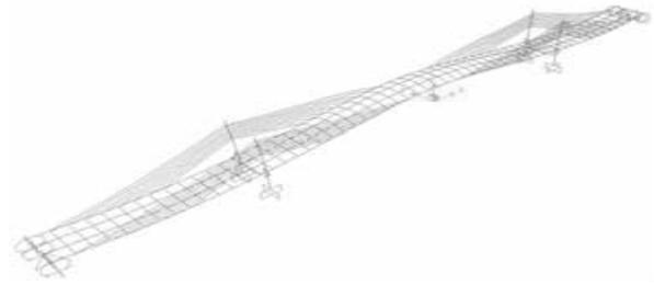
**Figure 6:** Mode 1 for span 75+150+75, T=1.09s
