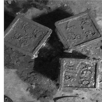
**Figure 1: Cubes casted with Dolomite Rock Sand**
