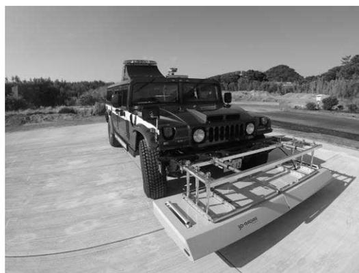
Figure 1: Ground Penetrating Radar-Mounted Vehicle
