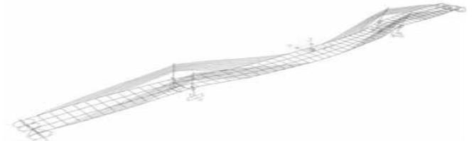
**Figure 7:** Mode 2 for span 75+150+75, T=0.87s
