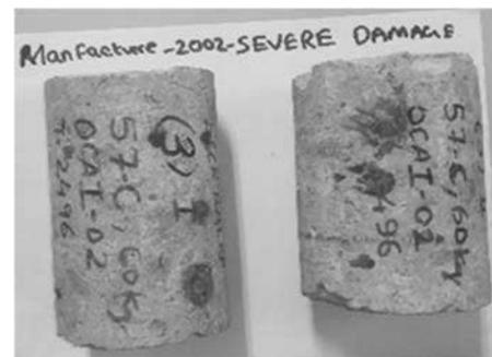
**Figure 5:** Core samples of "Severe damage" sleepers
