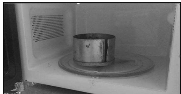
**Figure 1:** Microwave oven with single split mould
