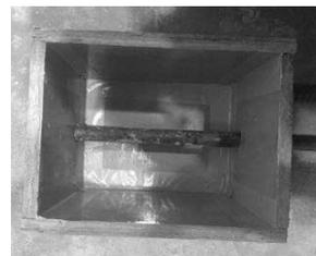
(b) Formwork of corroded reinforcement specimen
