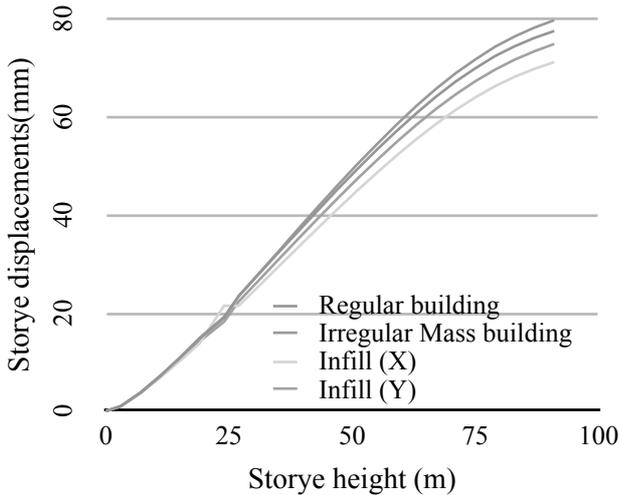
**Figure.7.** Storey displacements (max) of Regular building and Building having mass irregularity including the effect of infill wall stiffness.
