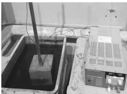
**Figure 3:** Corrosion acceleration test
