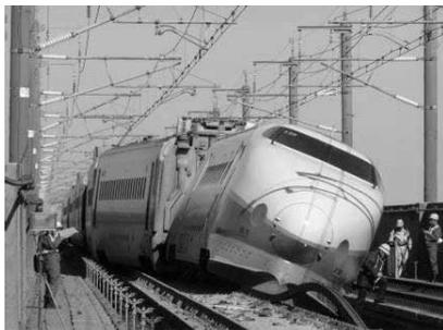
**Figure 1:** Shinkansen derailed by earthquake
