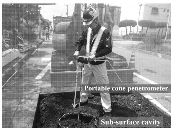
Figure1: Portable cone penetration test
