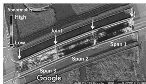
Figure 2: Example of Signal Processing Result
