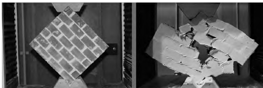
Figure 4: URM and P1-F after the tests
