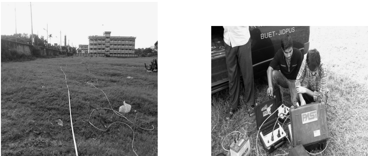
Figure 15: Spread of electrodes and ERT arrangement during resistivity test
