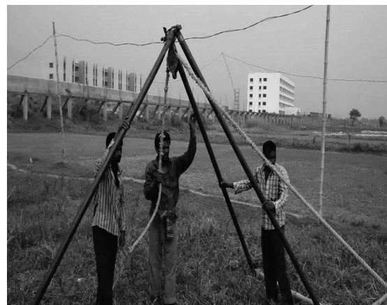
Fig 19: Using 140lb hammer as impulse source
