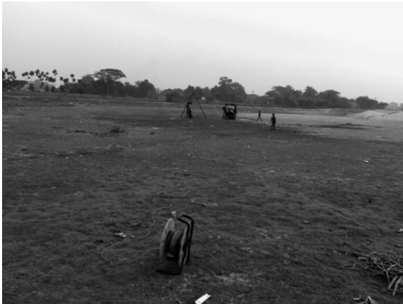
Fig 14: Spread of geophones during refraction test at Vatara
