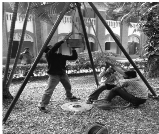
Fig 7: Using 140lb hammer as impulse source
