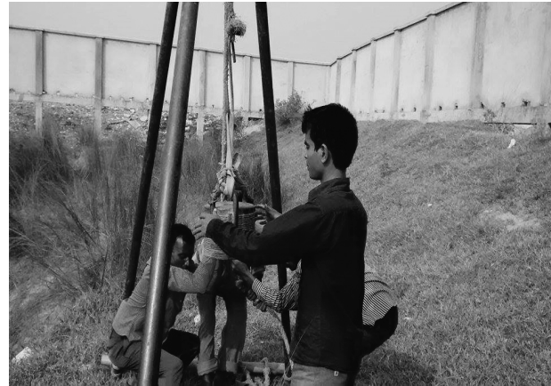
Fig 11: Using 140lb hammer as impulse source
