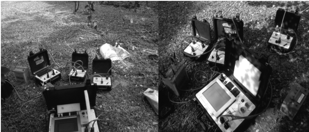
Figure 17: Spread of electrodes and ERT arrangement during resistivity test
