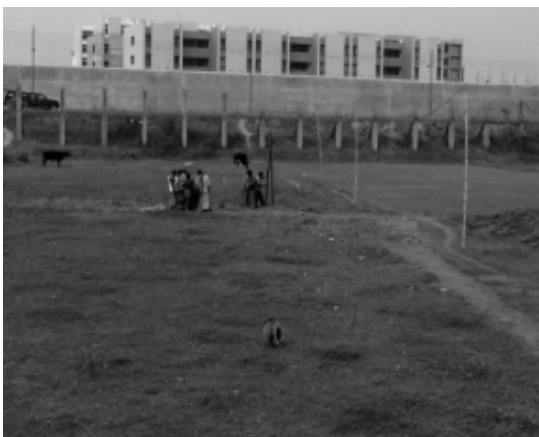
Fig 18: Spread of geophones during refraction test at New Jail
