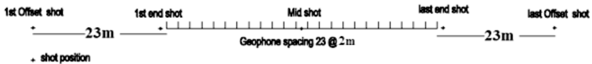
Fig 8: Layout of shots position during seismic refraction test at BUET
