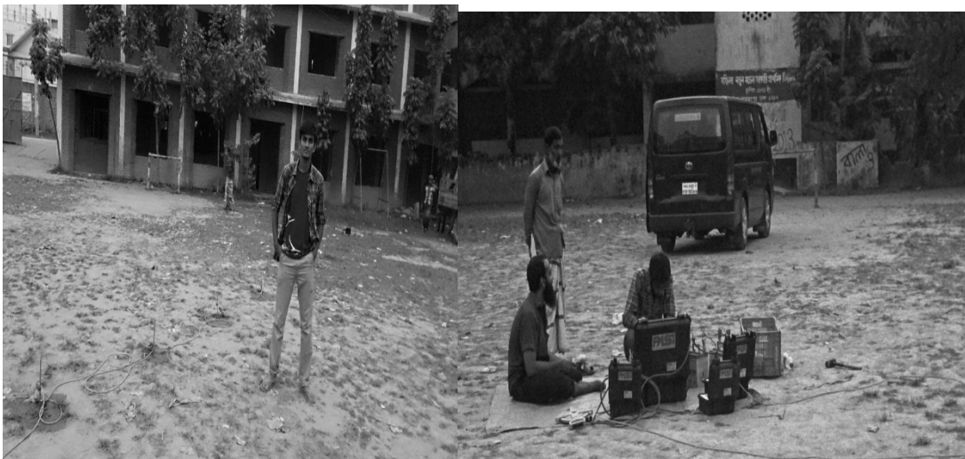
Figure 13: Spread of electrodes and ERT arrangement during resistivity test
