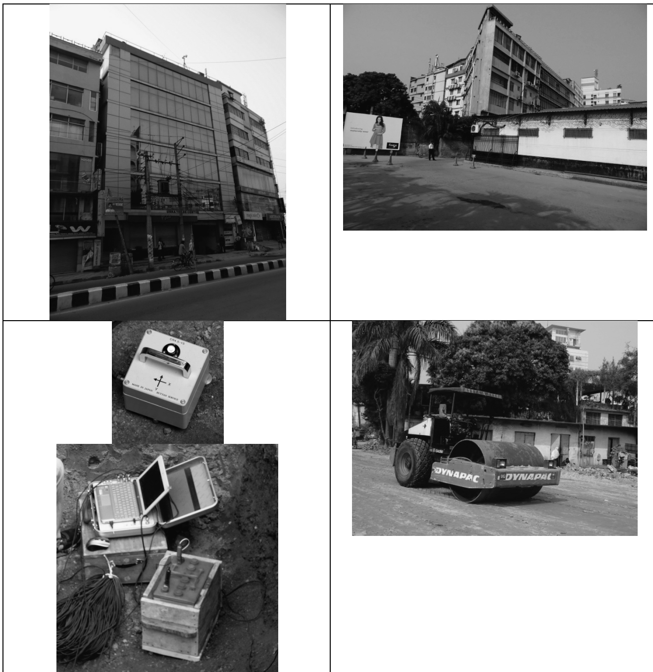
Figure 2 Measurement of building vibration using Microtremor observation system
