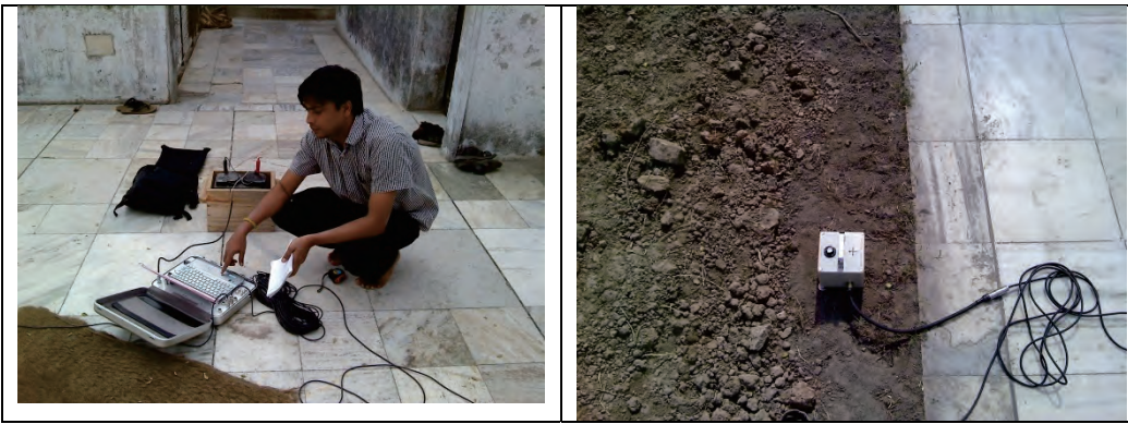
Figure 3: Data collection by Microtremor
