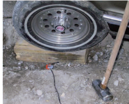
Figure 2: Wooden Plank Source Used In Downhole Seismic Test
