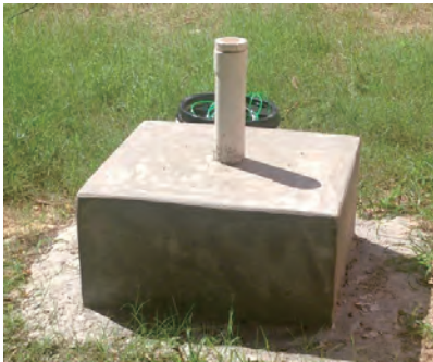
Figure 1: PVC pipe cased borehole.
