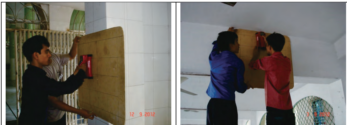
Figure 6 : Ferroscan observations of Column and beam
