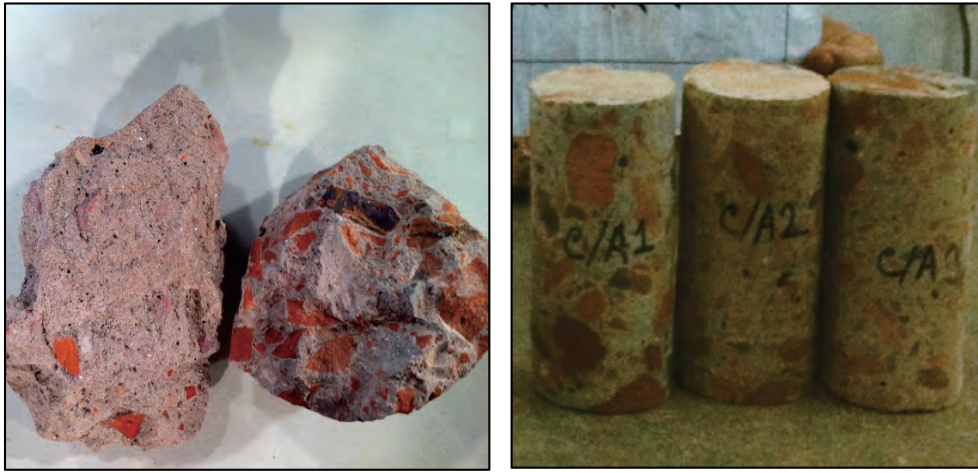
Figure 3. (a) Broken samples collected from the building site and (b) Concrete cores collected from beams, columns and slabs of the collapsed building
