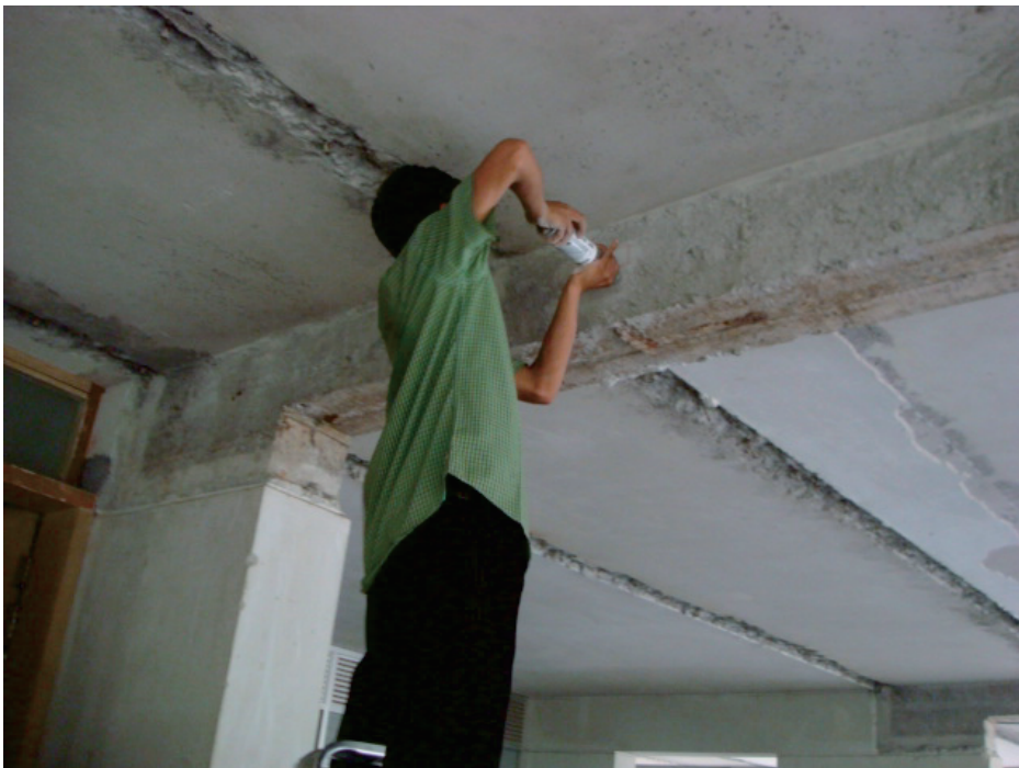
Fig. 2 Use of Schmidt Hammer to estimate concrete strength
