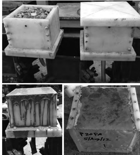
Figure 4: Compressive Strength specimen preparation through pumping
