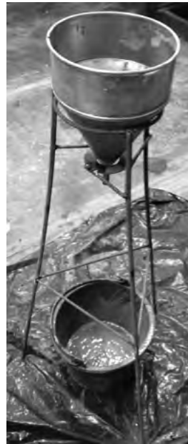
Figure 1: ASTM C939 Flow Cone
