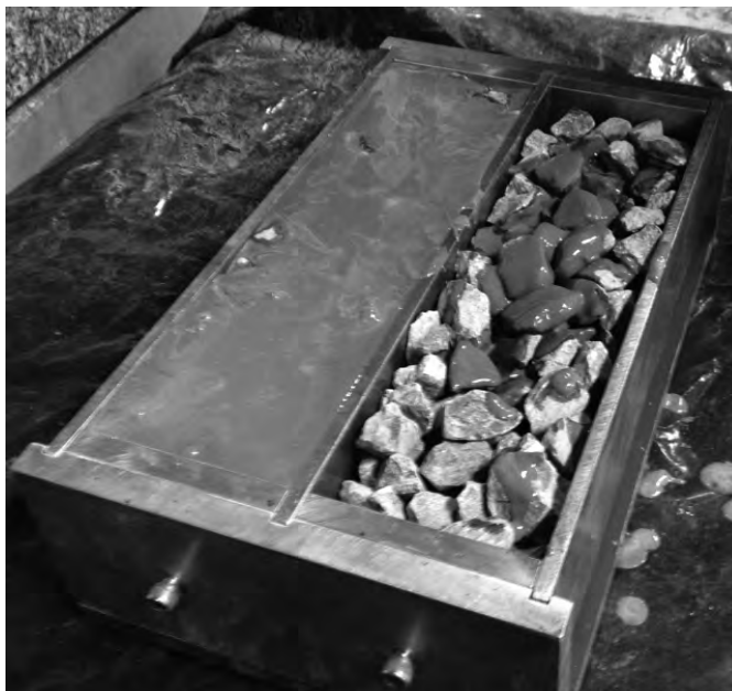
Figure 5: Shrinkage Specimen preparation using PA method
