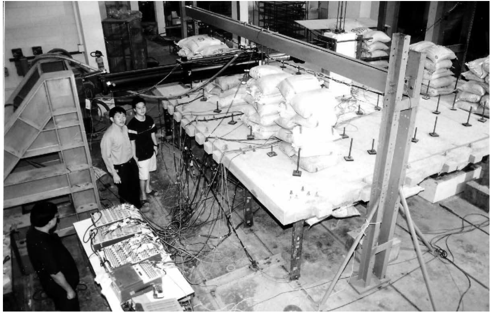
Figure 4: Setup for reversed cyclic loading test
