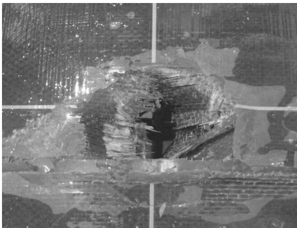
Figure 2: Appearance of FRP panels after failure
