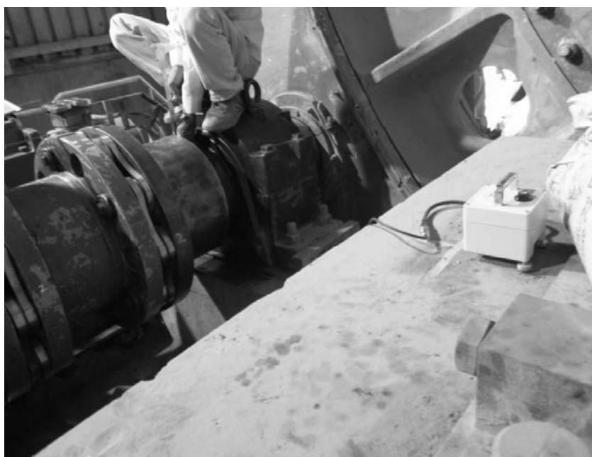
Fig. 2 Measurement of Plant Vibration using Microtremor System
