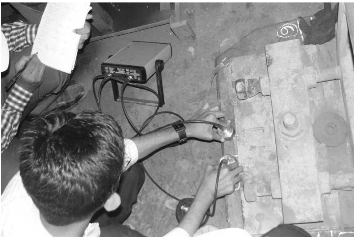
Fig. 2 Use of Schmidt Hammer to estimate concrete strength at the Inlet foundation and use of UPV to detect cracks on the top of gear box
