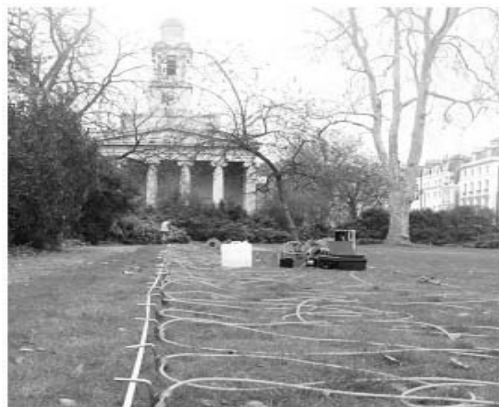
Figure 7: A typical resistivity imaging survey, above comprises an array of ground electrodes connected to a resistivity meter. The length of line determines the depth penetration and resolution of the data.
