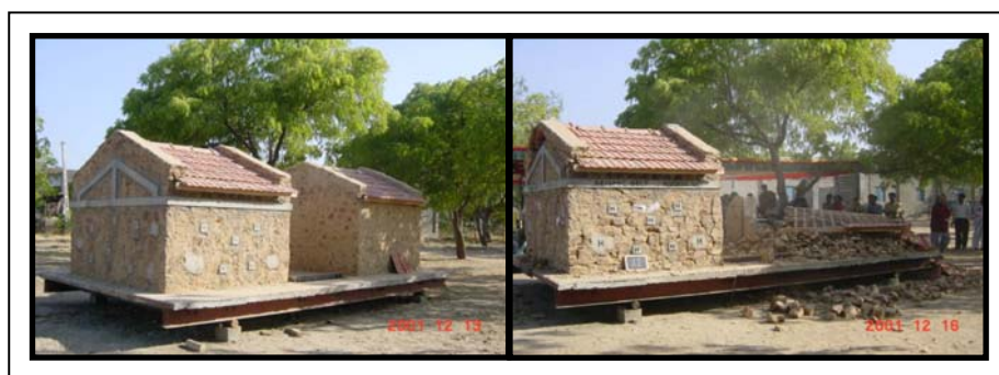
Figure 4: Shake table testing with rural construction
