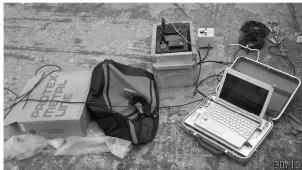
Figure 4: Test equipments used in microtremor measurements.
