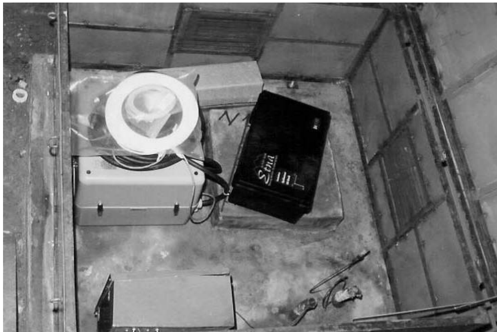
Figure 1. Free field ETNA Instrument Setup
