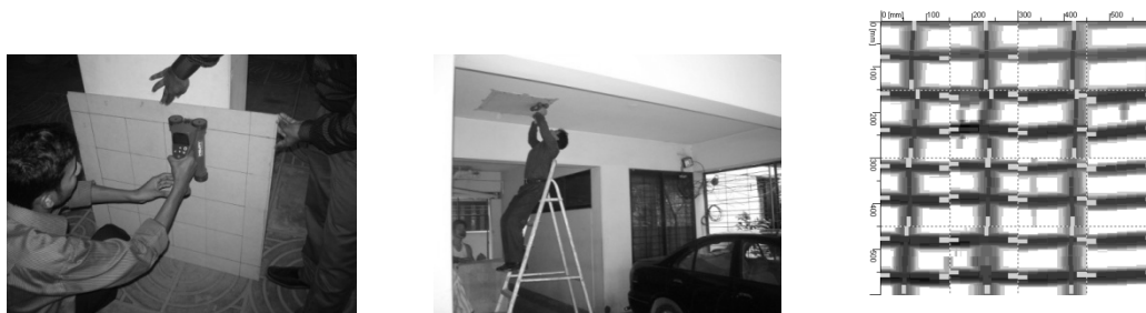
Figure 3(b): Column and slab checking using Ferrosan
