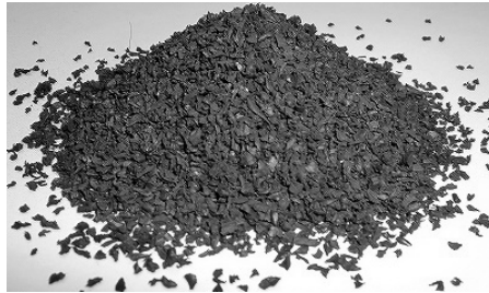
Figure 5.1 Rubber crumbs (size 1 to 3 mm) from recycled rubber tires
