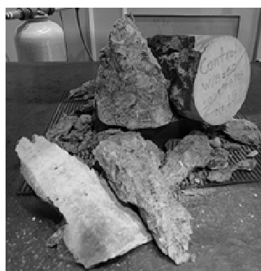
Figure 5.7 Failure mode of normal concrete under compressive loading
