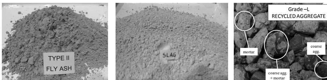
Waste and recycled materials used in concrete: fly ash (left), blast furnace slag (middle), and recycled aggregates (right)
