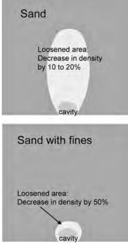
Typical patterns of cavity and loosened area developed in sandy ground
