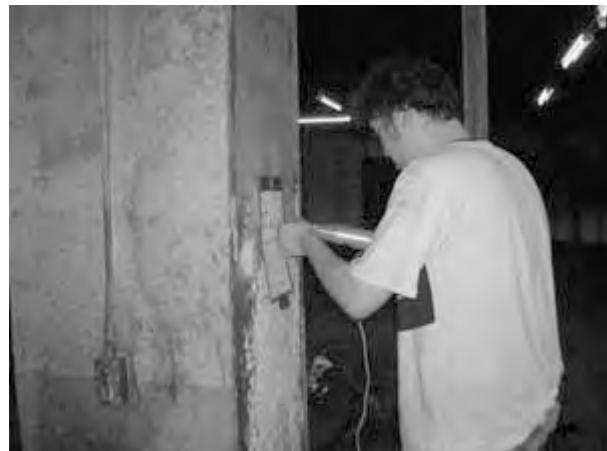
*Figure 3: Testing of the surface hardness of columns by Schmidt hammer*
