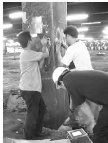
*Figure 4: Measurement of ultrasonic wave on columns*
