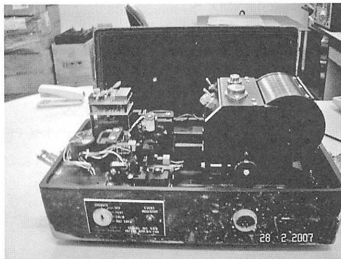
Figure 2 Photograph of SMA-1 Strong Motion Accelerograph
