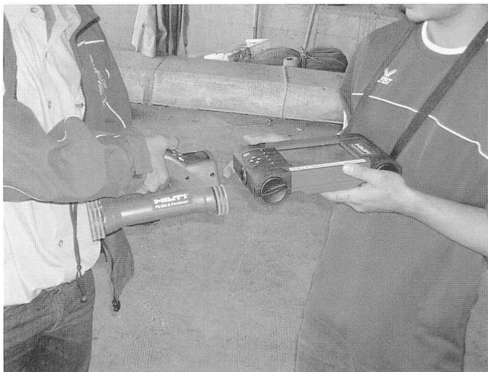
Figure 21: Transferring measured data of covering depth
