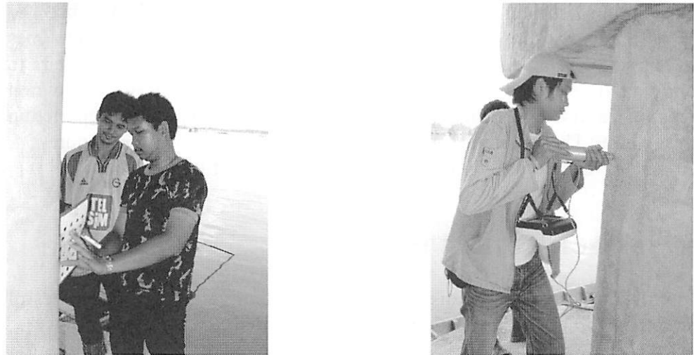
Figure 32: Method of conducting Schmidt hammer
