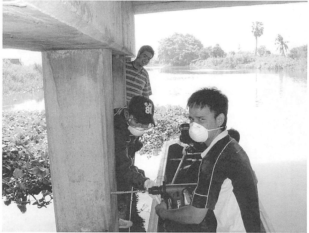
Figure 25: Collecting concrete powder sample
