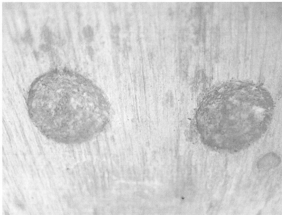
Figure 42: Observation of carbonation at very small distance from surface
