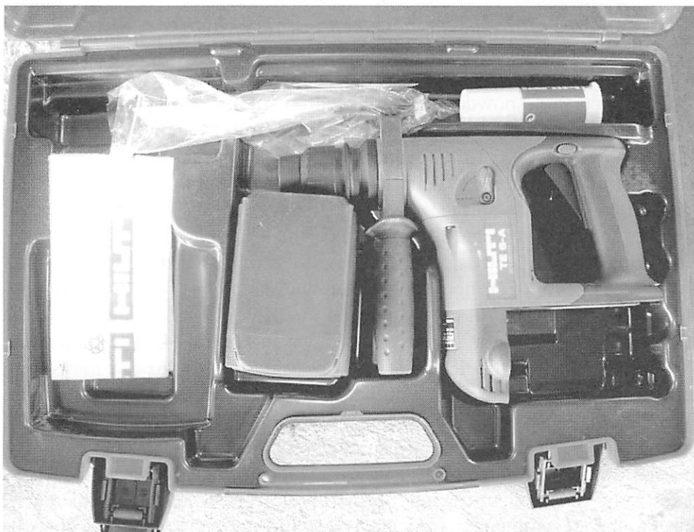
Figure 23: Portable drilling machine with 14mm drilling bit
