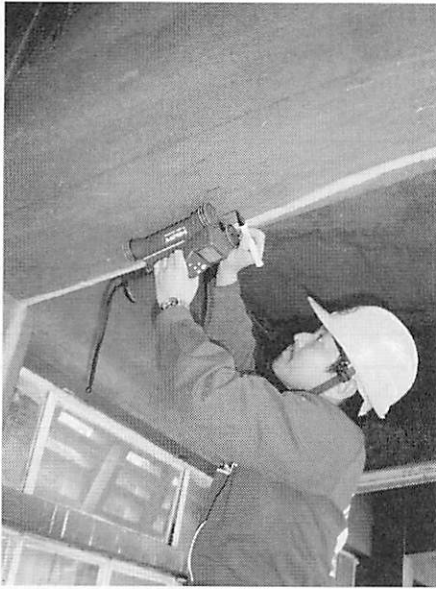
Figure 23(a) Beam reinforcement detection with Ferroskan at Architecture building
