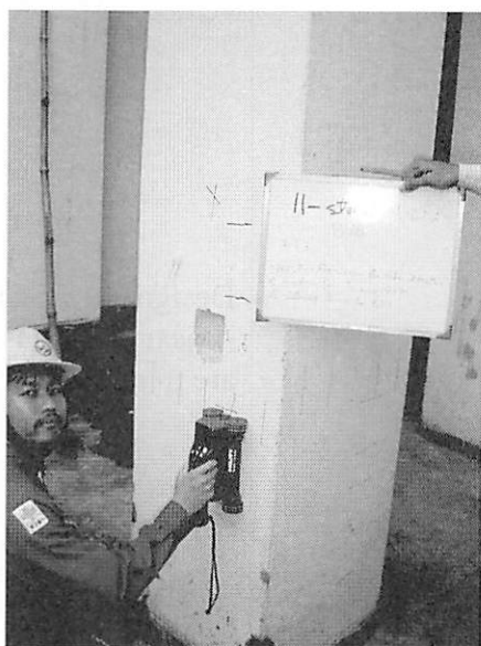
Figure 13(a) Column reinforcement detection with Ferroskan at 11 story Tower building.
