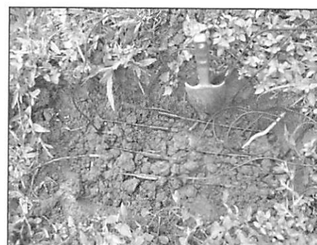
Probes installed at 10 cm depth
