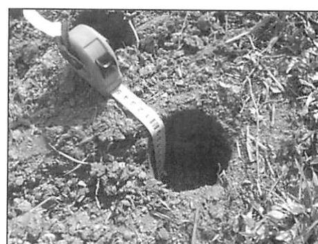
Hole to take sample to estimate actual volumetric soil moisture
