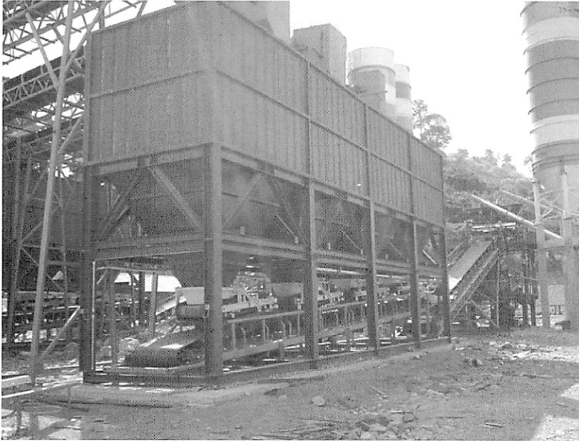
Figure 29: Mixing plant capable to continuously mix concrete
