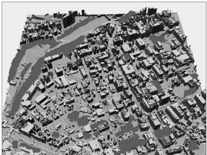
Three-dimensional expression of bird's-eye view of a city made by laser scanner
