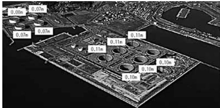
Sloshing wave height in all tanks estimated by the proposed system
