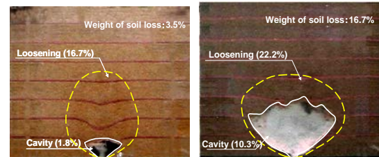
Generation and expanding process of cavity and loosening in the ground
