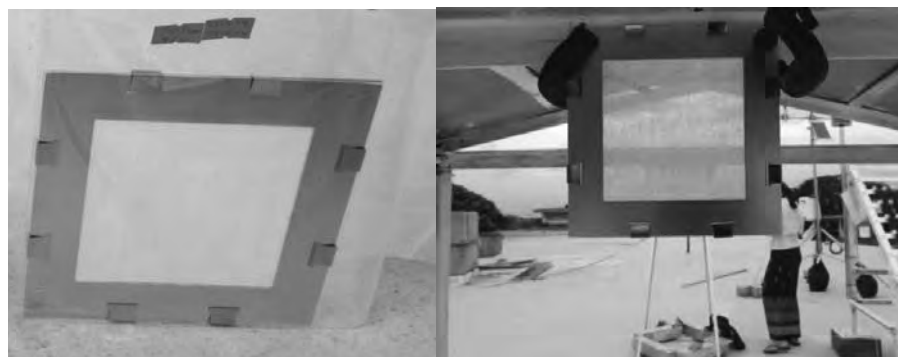
Figure 2: Testing for chloride with dry gauze methodology
