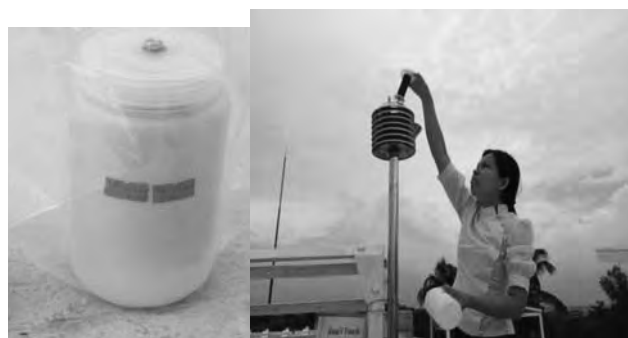
Figure 3: Testing for sulfur with cylinder methodology
