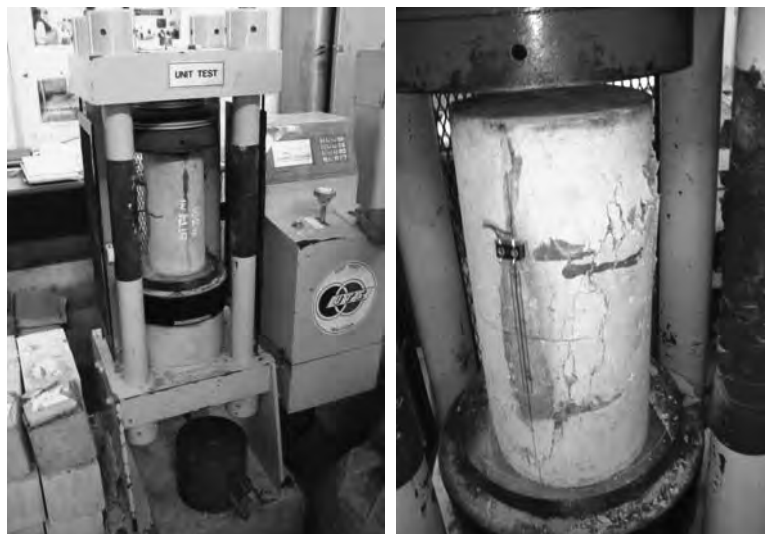
Figure 4: Concrete compression test
