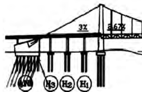
Figure 16 Reinforcement with skew piles
