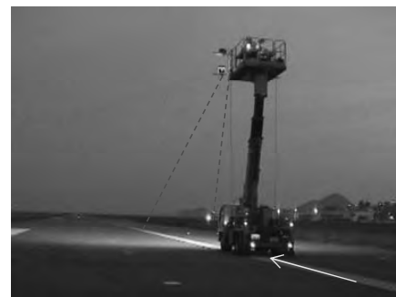
Figure 18: The inspection by Infrared Imaging Camera
