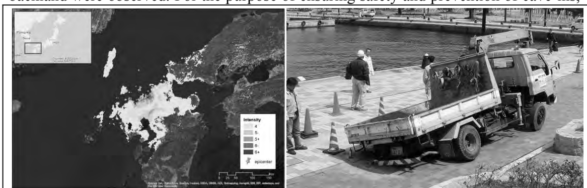
Figure 6: I_{jma} map of 2005 Fukuoka Earthquake and a picture taken at the time of recovery work showing pier floor cave-in.
