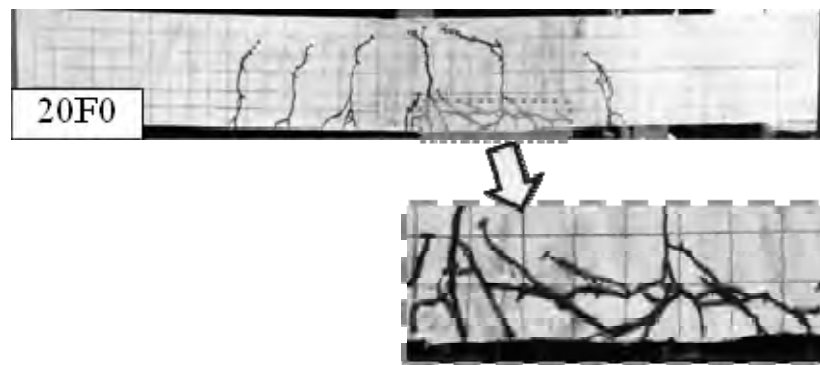
Figure 9: Crack pattern of specimen 20F0 at failure
