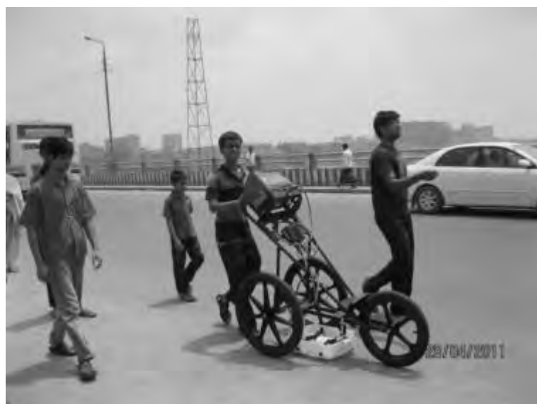
Figure 3: GPR data collection
