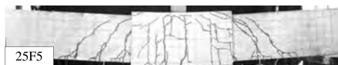
Figure 10: Crack pattern of specimens retrofitted by ferrocement jacket
