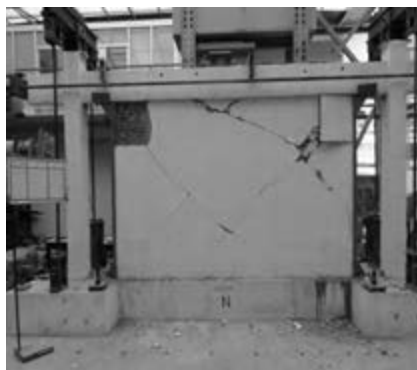
Figure 4: Retrofitted masonry-infilled RC frame (MIRCF02) with the innovative scheme at 2% drift (test terminated for safety reason)
