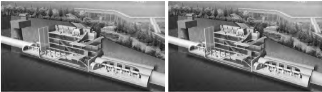
(a) Common station (excavation + tunnel type)
