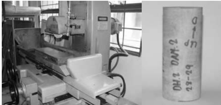
Figure.5 Rock sample preparation for rock mechanic testing
