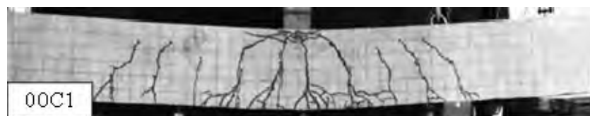
Figure 8: Crack pattern of specimen 00C1 at failure
