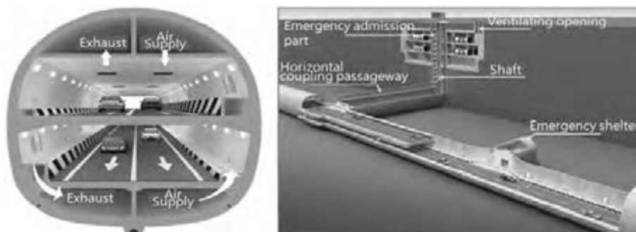
Figure 5 Ventilation method and emergency evacuation facility
