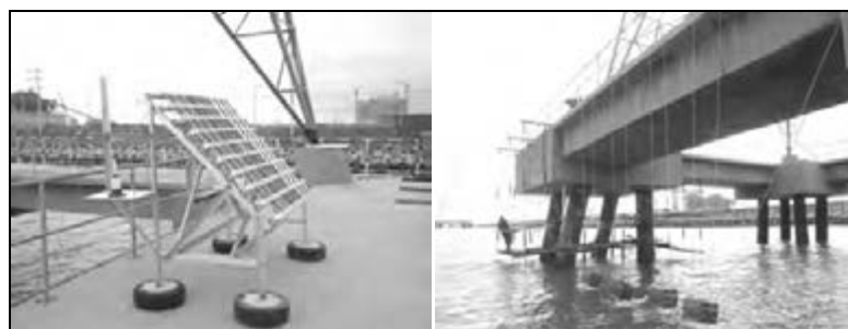
Figure 2: The exposure rack of atmospheric zone (left) and tidal zone (right)
