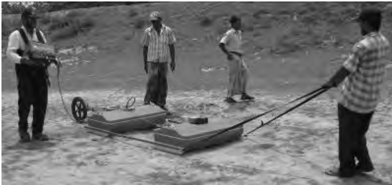
Figure 4: Diagram of the transmit (Tx) and receive (Rx) antennas, airwave, waveguide dispersive modes, and refraction (Top). 100-MHz antennas with fiber optic circuitry to trigger the receiver and antennas on the study line (bottom).
