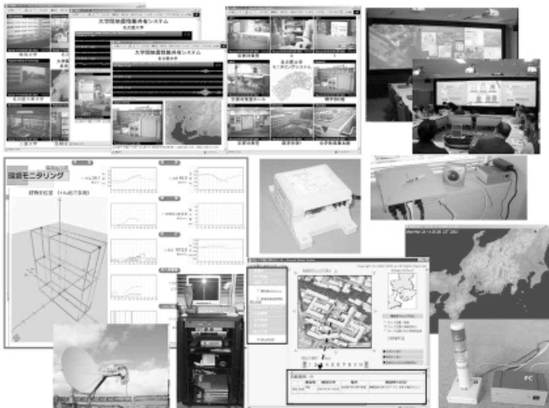
Earthquake disaster information system at Nagoya University. This system combines cameras and seismometers to monitor the disaster situation in real-time at Nagoya University and surroundings.
