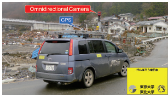
Sensing vehicle equipped with omni-directional camera
