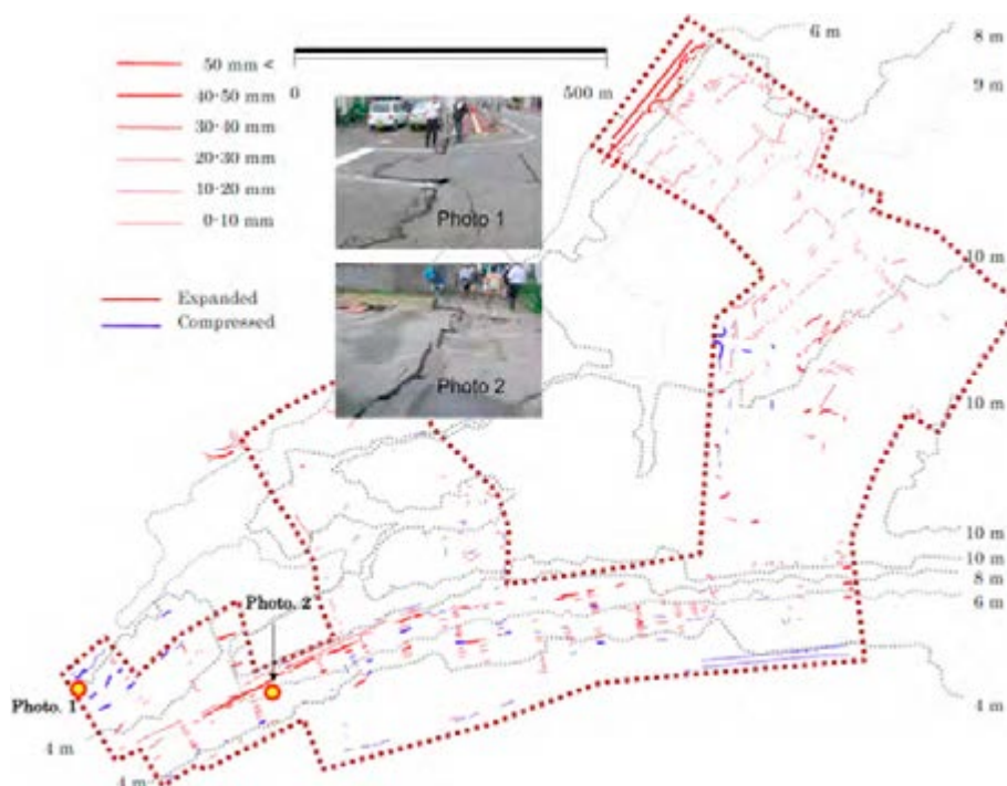
Figure 2: Pavement Cracks of the Kashiwazaki City Downtown
