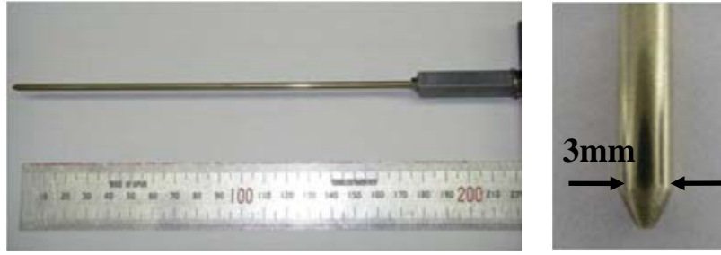
Figure.2 Penetration needle and tip shape
