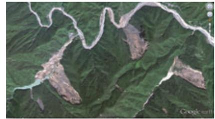
***A rash of landslides and the resulting formation of natural dams at Nagatono and Akatani in the Kii mountain range due to a large amount of rainfall caused by Typhoon Talas.***
