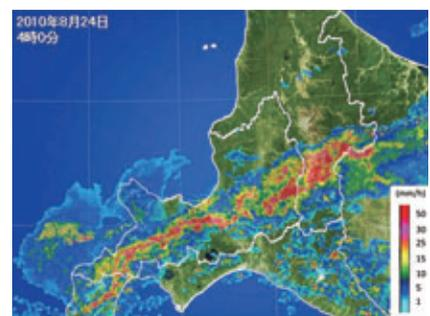
*Distribution of rainfall per hour on August 24, 2010. The rain area illustrated in red is a line-shaped rain band which caused the heavy rainfall along the Chubetsu River.*
