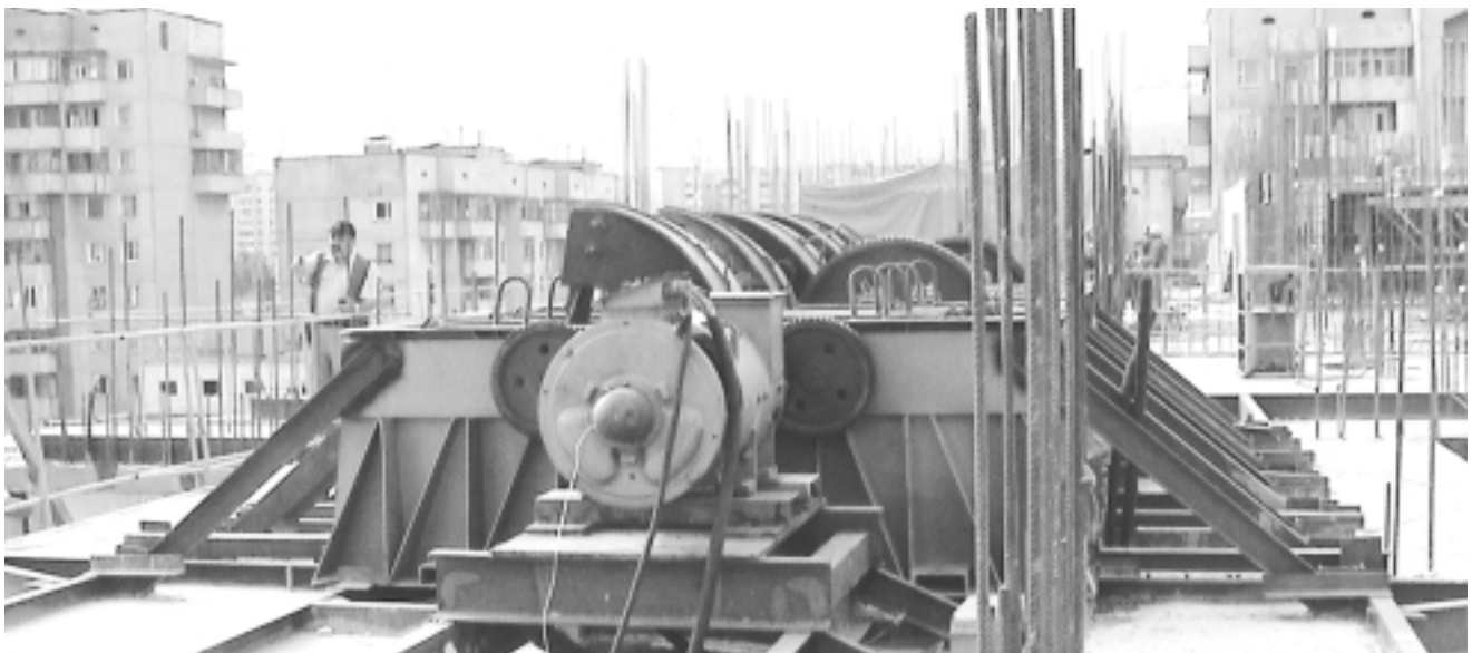
Shaking test of actual 7-story apartment house at the Almaty city
