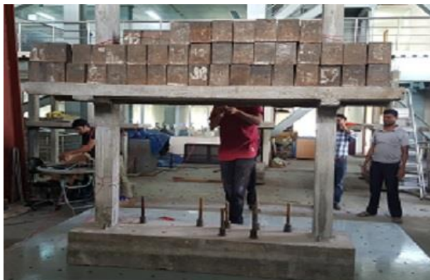
RC frame without and with BRB on the BUET-JIDPUS Shaketable
