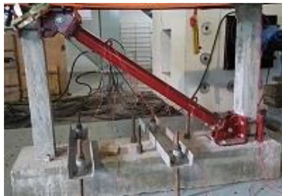
RC frame without and with BRB on the BUET-JIDPUS Shaketable
