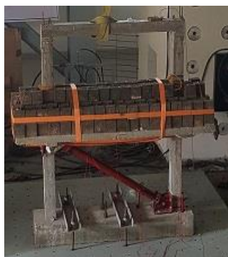
RC frame without and with BRB on the BUET-JIDPUS Shaketable
